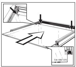
■ Push the middle pane into the frame almost to the end. The material (M-) number printed on the pane must be legible in the bottom right hand corner (see illustration). Fit the sealing strip into position, then push the pane in as far as it will go.
